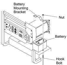
Figure 9 - Battery Hold-Down System (Model PGH7500IE Shown)
